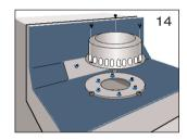
2.7 Screw the strainer (with gravity flow) or cover (with pressure flow) using the enclosed fastening screws to the loose flange (Fig. 14).
