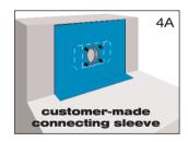
1.4 Spread the connecting sleeve ready-mounted at the factory (DN 70 and DN 100 versions) or the connecting sleeve made by the customer (DN 50 version) consisting of **bitumen/EPDM compound** or of **plastic**, and attach it to the substrate (Fig. 4 or 4A). Do not allow creases to form. On the DM 50 version make 14 mm holes in the connecting sleeve with a hole punch for the threaded bolts to pass through. The loose flange can be used as a template.
