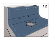
2.5 Unroll the second layer of the **roof sealing sheet** over the drain. Use a hole punch to make 14 mm diameter holes in the roof sealing sheet for the threaded bolts to pass through. The loose flange can be used as a template (Fig. 12). Roll back the second layer of the roof sealing sheet, weld the connecting sheet and the second layer of the roof sealing sheet in accordance with the laying instructions from the manufacturer of the roof sealing sheet.
