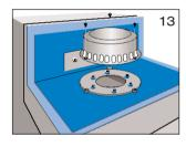
3.6 Screw the strainer (with gravity flow) or cover (with pressure flow) using the enclosed fastening screws to the loose flange (Fig. 13).
