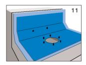
2.4 Cut the **connecting sheet** of the existing roof sealing sheet, with a size of 700 mm x 1000 mm to length on site (Fig. 11).
