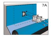
1.8 With the DN 50 version, place a compression seal over the vapour barrier sheet, and clamp with loose flange and included screws (Fig. 7A). Tighten the enclosed screws using an SW 17 open-ended or ring spanner, working criss-cross. Tightening torque: 20 Nm (bituminous vapour barrier sheet) or 30 Nm (plastic vapour barrier sheet).
