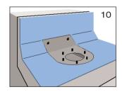
2.3 Unroll the first layer of the **roof sealing sheet** over the scupper drain, and make a cut-out in the region of the fixed flange (Fig. 10).
