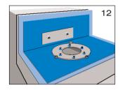
3.5 Clamp the connecting sheet with loose flange and the included screws (Fig. 12). Tighten the enclosed hexagonal flange nuts with an open-ended or ring spanner SW 15, starting at the flange side under 90°. Then tighten the remaining hexagonal flange nuts, working criss-cross. Tightening torque: 30 Nm.
